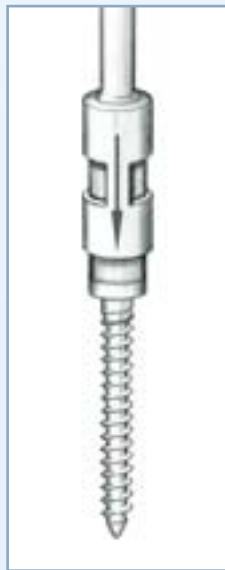
Fig. 5: Monoaxial screwdriver assembly
