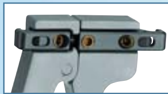
Fig. 22: Placement of the cross connector in the cross connector bender FW203R
