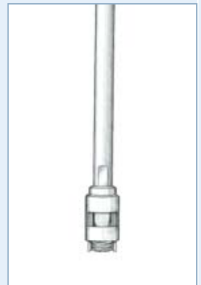
Fig. 14: Fully engaged set screw
