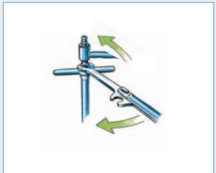
Fig. 38: Tightening the nut with 15 Nm FW331R
